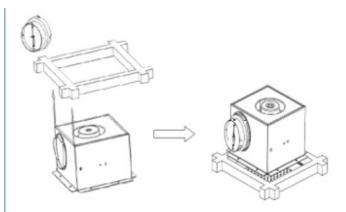
**Step 3**: Align the duct connector with the directional arrow (indicating airflow path) and lock it onto the cabinet's exhaust port using a twist-to-lock system for airtight sealing.
