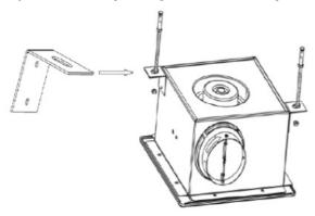
Step 2: Attach the fan enclosure or housing unit to the pre-assembled frame, securing it with vibration-dampening fasteners.
