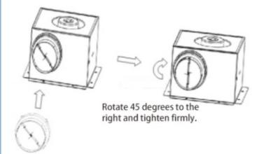
Fasten the air duct interface to the air inlet and outlet.
