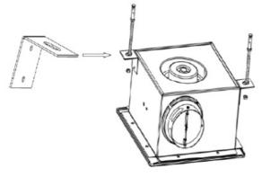
2. Firmly affix the storage unit (or enclosure) to the pre-installed frame.
