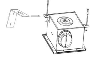
2. Firmly affix the storage unit (or enclosure) to the pre-installed frame.
