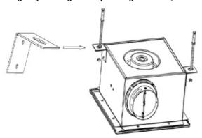
2. Firmly affix the storage unit (or enclosure) to the pre-installed frame.
