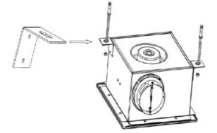
2. Firmly secure the storage unit (or enclosure) to the pre-installed frame.
