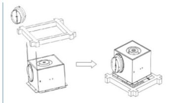
3. Carefully line up the ventilation duct connector with the arrow direction indicated and securely attach it using a twist-lock mechanism to the designated air outlet port on the cabinet, ensuring proper airflow connection.
