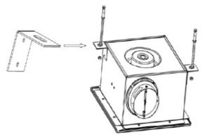
2. Firmly affix the storage unit (or enclosure) to the pre-installed frame.
