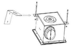
2. Firmly affix the storage unit (or enclosure) to the already installed frame.
