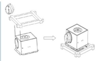
3. Carefully align the ventilation duct connector with the arrow direction indicated, and firmly secure it using the twist-lock mechanism to the designated air outlet port on the cabinet. This ensures an accurate and efficient airflow connection.
