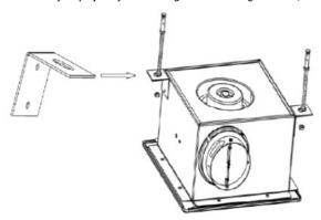
2. Secure the storage unit or enclosure firmly to the pre-installed frame, ensuring a stable and reliable installation.
