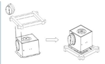
3. Align the ventilation duct connector with the arrow direction indicated and firmly attach it using a twist-lock mechanism to the specified air outlet port on the cabinet, ensuring correct airflow connection.
