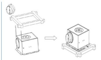
3,Align the air duct connector with the arrow direction and twist-lock it onto the air outlet of the cabinet.
