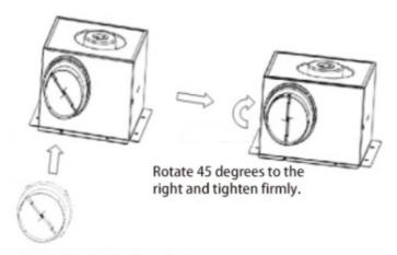
Fasten the air duct interface to the air inlet and outlet.
