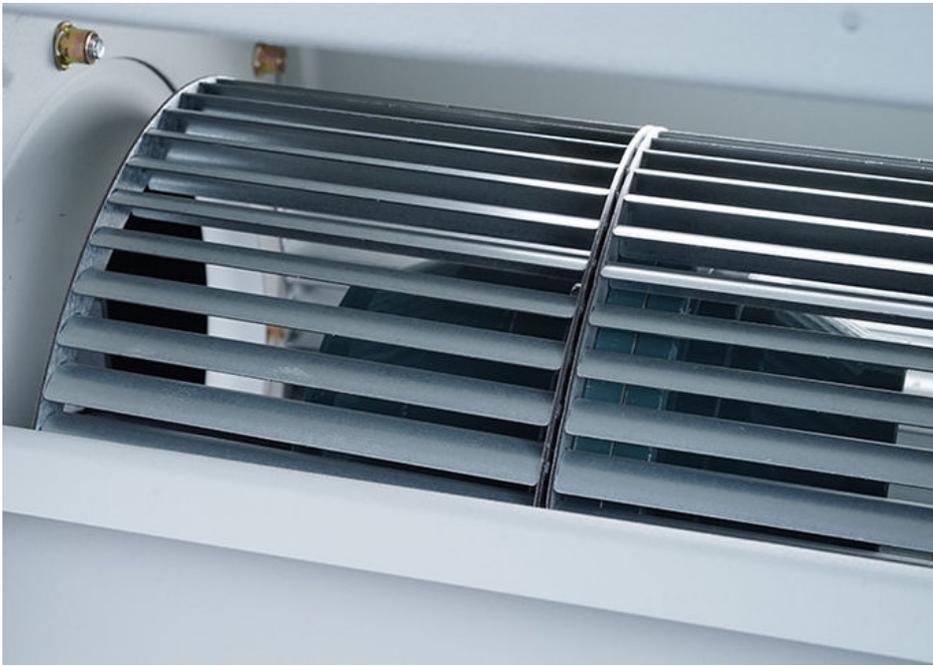
**Motor:** Utilizes a three-phase asynchronous, low-noise external rotor motor. The impeller's central disc is directly mounted on the motor housing, allowing the fan speed to be adjusted using a three-phase voltage regulator or a variable frequency drive to meet the varying demands of system load.
